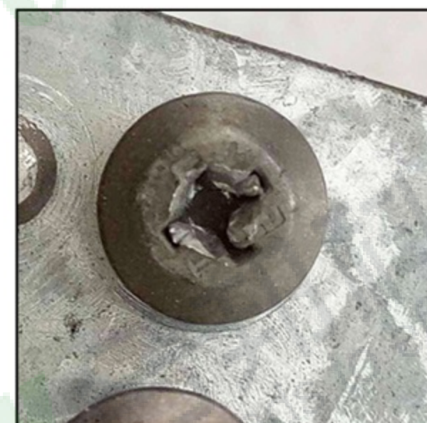
头部驱动滑脱 Socket slide
